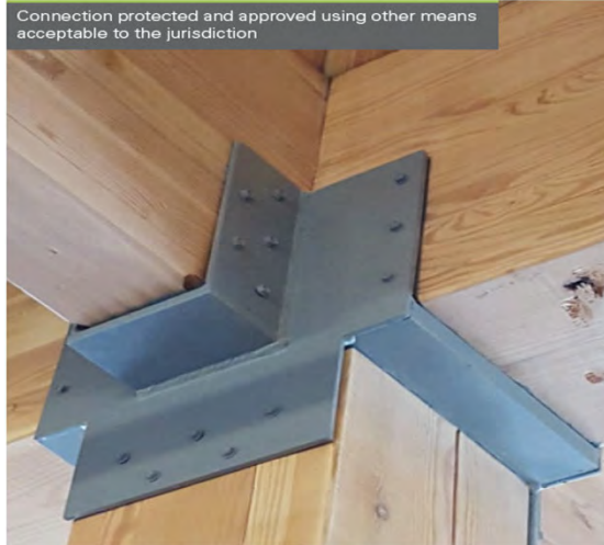
Exposed side of an assembly prior to a fire test
